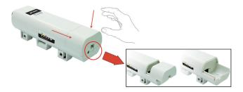
2. Plug a standard Ethernet cable into the RJ45 port.
