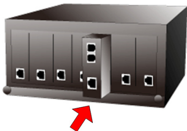
Figure 3-6: Insert a VDSL2 converter into an available slot
