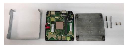
7. Remove the board, can keep the power line connected.
