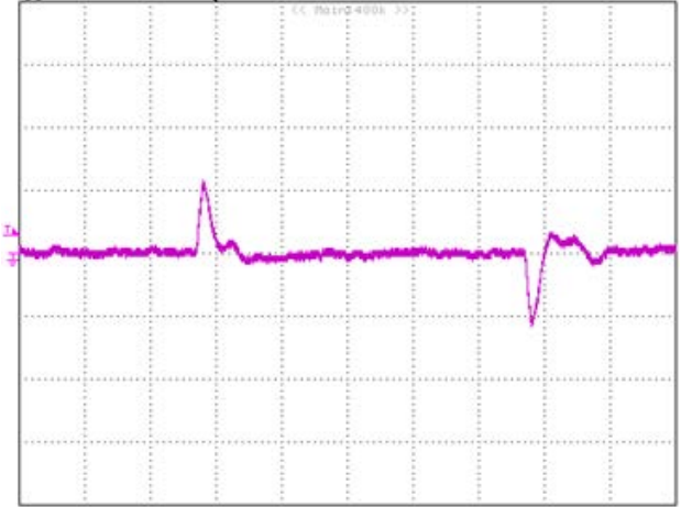
Figure 28: Output voltage response to step-change in load current (25%-75%-25% of 100A load at V_{in}=12V V_o=3.3V ; 100mV/div, 200uS/div, di/dt = 2.5A/\mu s ; 2000uF ceramic C_{out} )
