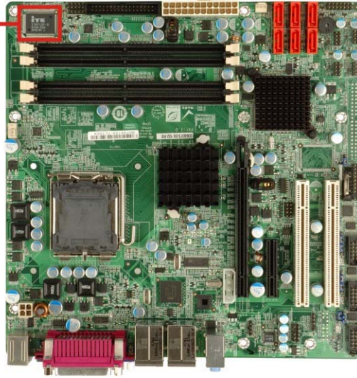
Figure 2-17: ITE IT8712F Super I/O
