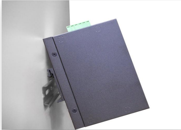
Figure 3.2 Insert the Switch on the DIN-Rail
