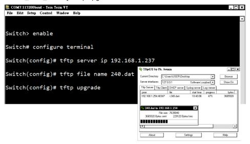
Fill in the TFTP server IP and upgrade file name behind the "tftp server ip [IP\_ADDRESS]" and "tftp file name [UPGRADE\_FILE\_NAME]"
