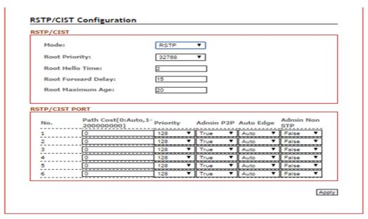
Figure 5.30 - RSTP Configuration Interface
