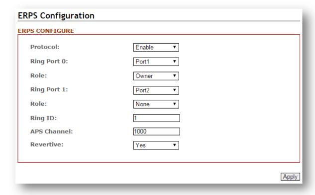
Figure 5.18 - ERPS Configuration Interface
