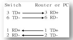
Figure 2.4 Straight-Through Cable Schematic
