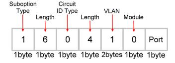
Figure 5.60 - DHCP Relay Option 82 Circuit ID
