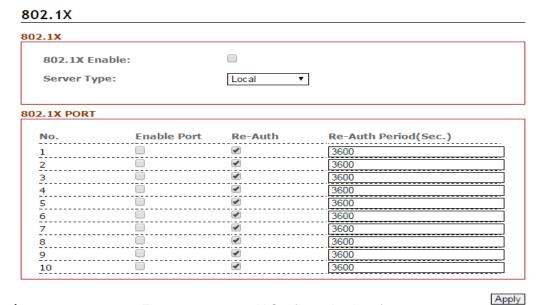
Figure 5.73 – 802.1X Configuration Interface
