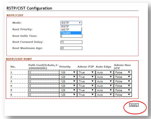
Figure 5.22 - RSTP/CIST Configuration Interface
