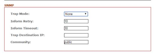
Figure 5.58 – SNMP Trap Setting
