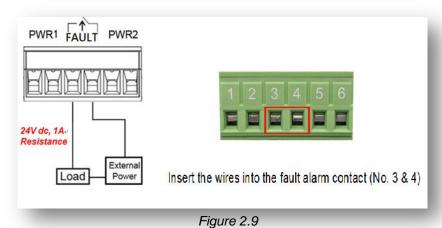
Wiring the Fault Alarm Contact
