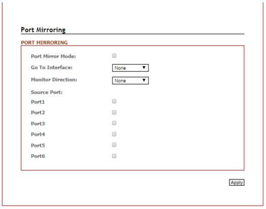
Figure 5.54 – Port Mirroring Configuration Interface
