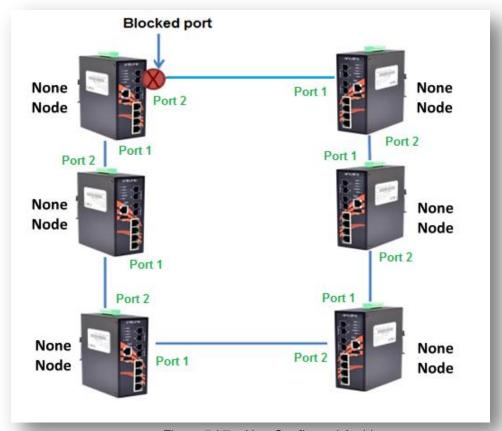
Figure 5.27 – Non-Configured Architecture
