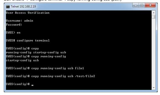
Fill in the folder and filename behind the "copy running-config usb" command.
