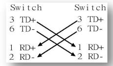
Figure 2.5 Crossover Cable Schematic
