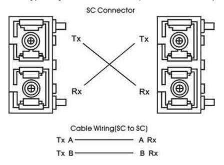
Figure 2.6 - Fiber Ports Connection
