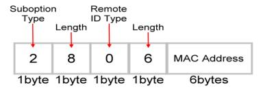
Figure 5.62 - DHCP Relay Option 82 Remote ID
