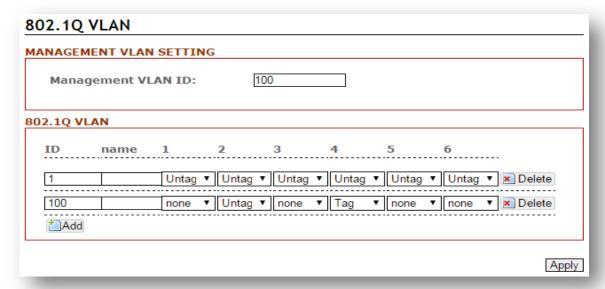
Figure 5.40 - 802.1Q VLAN Settings Interface
