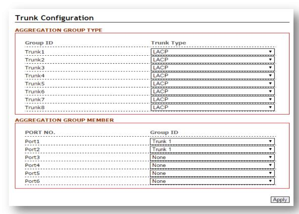
Figure 5.52 - Port Trunk Configuration Interface
