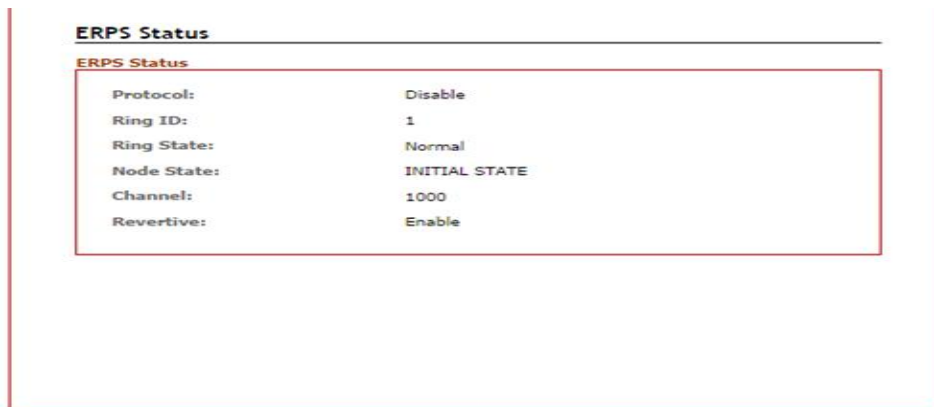
Figure 5.21 – Redundant Ring Network – ERPS Status
