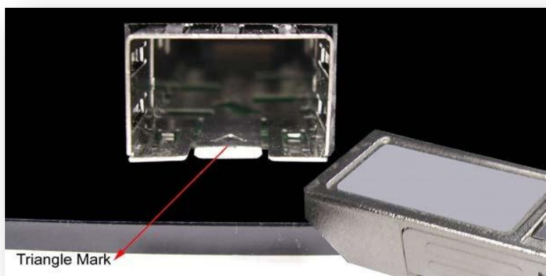
Figure 2.9 - Transceiver to the SFP Module
